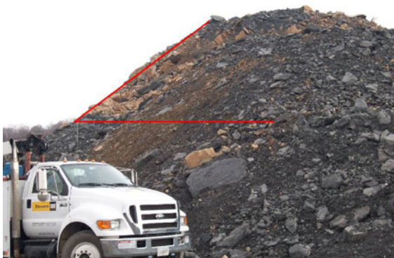
Fig. 5 Typical field determination of the angle of repose at National Site (White et al. 2009). Camera placed on a level and photo taken of material in loose state. Note the large number of oversize ( > 0.3 m) particles in the reclaimed material
