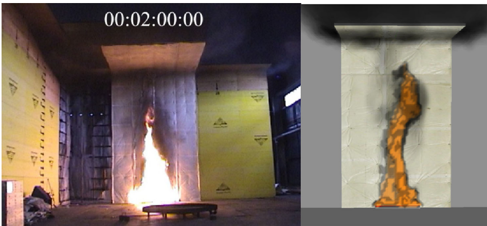
Figure 12. Test footage (left) and fire model visualization (right) 2 min into the test.
