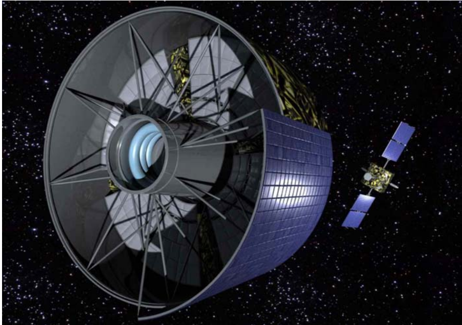
Fig. 1 The GRI mission deployed in space. GRI is composed of two spacecrafts flying in formation at a distance of 100 m. The optics spacecraft ( front ) carries the Laue crystal lens and the multilayer coated single reflection mirror payloads that concentrate incoming hard X-rays and soft gamma-rays onto a focal spot situated 100 m behind the spacecraft. The detector spacecraft ( back ), carrying the detector payload, is placed at the location of the focal spot to collect the concentrated photons
