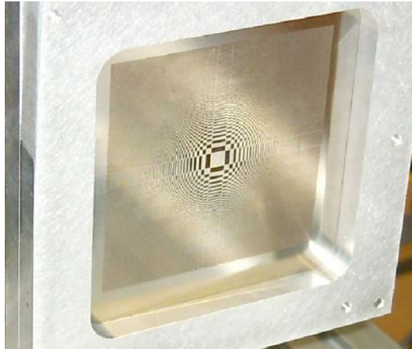
Fig. 4 Eighty millimeters square Fresnel primary array carved into a thin 80\ \mu\text{m} stainless steel foil, used for optical tests (58 Fresnel zones, 26,680 subapertures)
