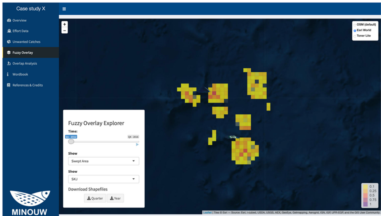
Fig. 7 Screenshot of the Fuzzy overlay panel, with an example from the case study of bottom trawl fisheries in the fictional case study near Palmyra Atoll. In this example, the different cells are coloured with respect to the (0–1) index scale in the bottom right side of the map
