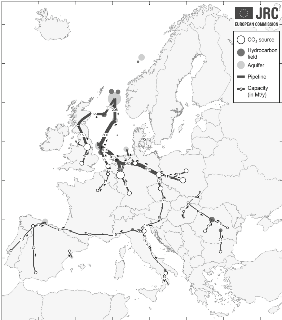
Fig. 3 CO 2 pipeline network in 2050, assuming joint international optimisation without participation of Denmark
