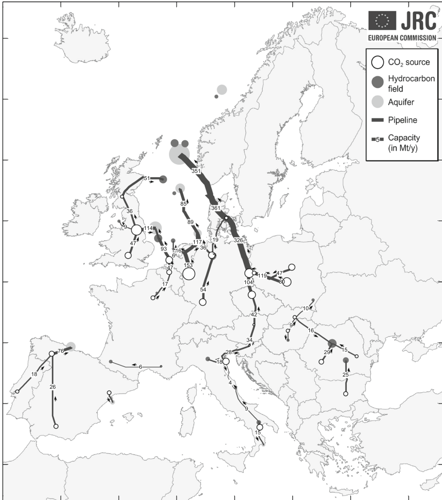
Fig. 1 CO 2 pipeline network in 2050, assuming joint international optimisation. Total amount of CO 2 captured and stored: 1,145 Mt/y
