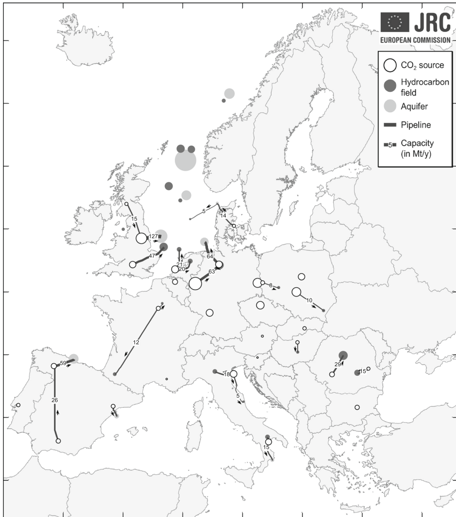
Fig. 2 CO 2 pipeline network in 2050, assuming individual optimisation per country, without international cooperation. Total amount of CO 2 captured and stored: 565 Mt/y
