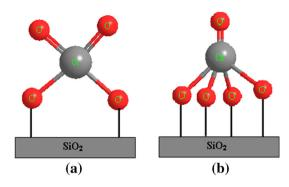
**Fig. 3** Schematic of molecular structures of "dehydrated" isolated surface CrO<sub>x</sub> sites on SiO<sub>2</sub> support (a) dioxo and (b) mono-oxo
