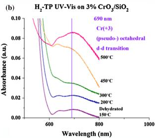
**Fig. 4** In situ  $\rm H_2$  TP–UV–vis DRS of 3 %  $\rm CrO_3/SiO_2$  (a) full spectrum and (b) zoomed in to see the  $\rm Cr^{+3}$  band. The 3 %  $\rm CrO_3/SiO_2$  catalyst was heated to 500 °C at 10 °C/min in 10 %  $\rm O_2/Ar$ , held at 500 °C for 1 h, and cooled to 150 °C. It was then flushed for 30 min in Ar. Then the temperature was ramped to 500 °C in 4.8 %  $\rm H_2$ . Spectra were taken every 50 °C
