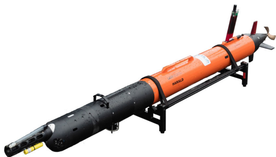
Fig. 9 The light AUV (Harald) produced by OceanScan was used in our experiments. The length of the AUV is 240 cm, and it is equipped with multiple sensors like CTD, Dissolved Oxygen, and Fluorometer
