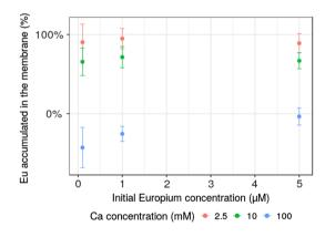
**Fig. 3** Eu accumulation within the cation-exchange membrane depending on initial Eu and Ca concentrations in the solution
