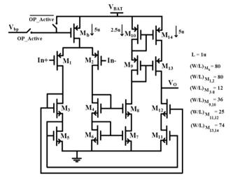
Fig. 11 OTA used in current sensor block
