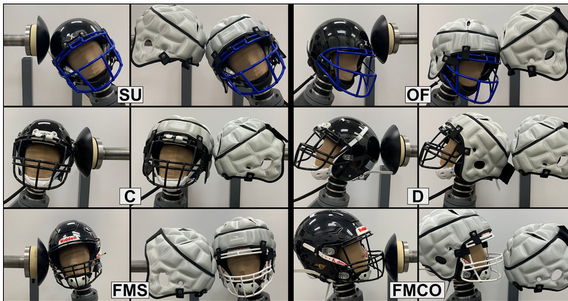
FIGURE 1. Helmet impact locations with and without the padded helmet shell cover affixed (SU = Side Upper; OF = Oblique Front; C = Side; D = Oblique Rear; FMS = Facemask Side; FMCO = Facemask Central Oblique). Examples of each helmet model tested are shown (top row = Xenith X2E+ ; middle row = Schutt Vengeance Pro LTD; bottom row = Riddell Speedflex Diamond).
