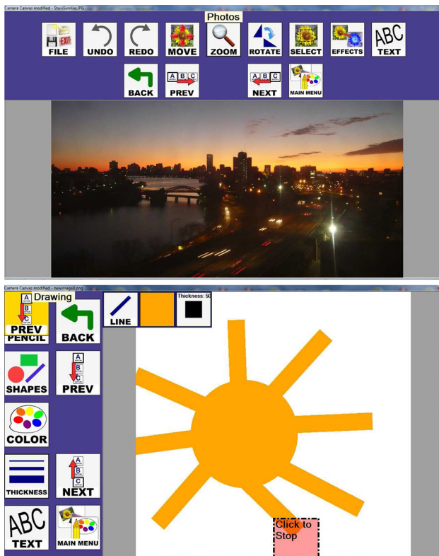
Fig. 1 Top Camera Canvas in Photo-editing mode with a horizontal-top layout and small buttons. Bottom Drawing mode with a vertical-left layout and larger buttons (right). The second set of Prev and Next buttons signify that the toolbar includes more buttons off-screen
