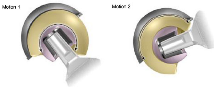
Fig. 1 The biomechanical concept of the dual mobility cup consists of a double articulation—between femoral head and liner and between liner and cup. The first motion occurs between the small femoral head and the inside of the polyethylene liner, until the neck of
