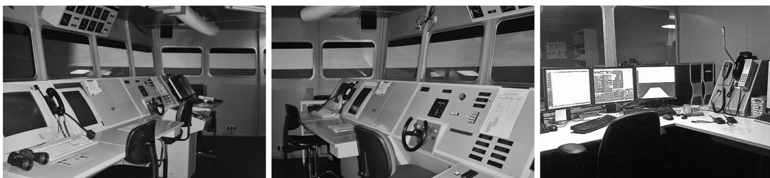
Fig. 2 Bridge simulator based on the ‘Van Tromp’ ship, seen from two angles and the trainer control room
