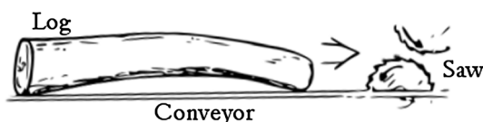
Fig. 1 Illustration of sawlog being sawn ‘horns down’
