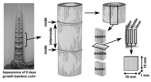
Fig. 1 Process of specimen preparation. In each internode, specimens were prepared to investigate the changes in cellulose crystallinity in cell walls along the longitudinal or radial directions
