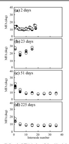
Fig. 6 Microfibril angle (MFA) in the radial position in bamboo cell walls in each growth period. *Black, gray, and white circles* indicate the results in the specimens prepared from *outer, middle, and inner* positions in each internode, respectively
