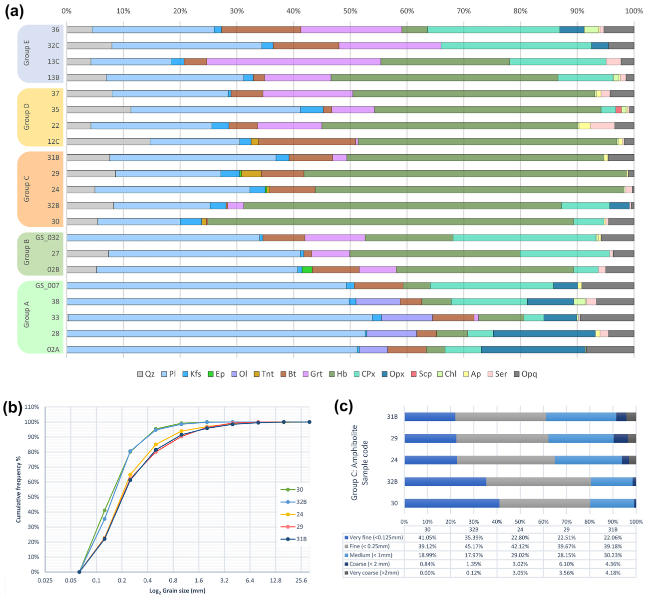
Fig. 8 Quantitative petrographic data. a Summary of mineral contents determined by point counting. Arrangement and color-coding of samples follow the subdivision of rock types in groups A–E. b Cumulative grain size distribution curves for samples in group C: Amphibolite. c Bar chart and data table showing the proportions of different grain sizes among the samples in group C
