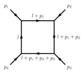
Fig. 1. Basic one-loop box diagram
