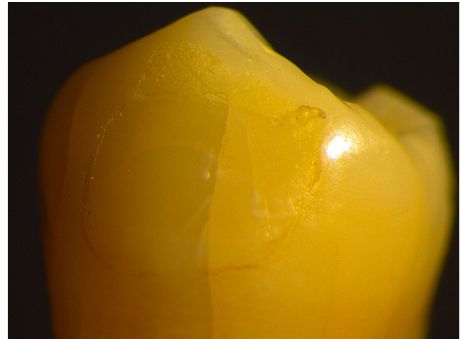
Fig. 7 Stereomicroscope image of specimen with an ARI score of 5
