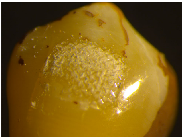
Fig. 4 Stereomicroscope image of specimen with an ARI score of 2
