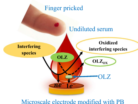
Fig. 1 Scheme of olanzapine detection in microliter volumes of undiluted serum samples using a platinum black-modified microelectrode
