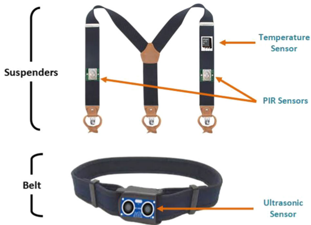
Fig. 5 Skeleton view of proposed suspender and belt equipped with sensor
