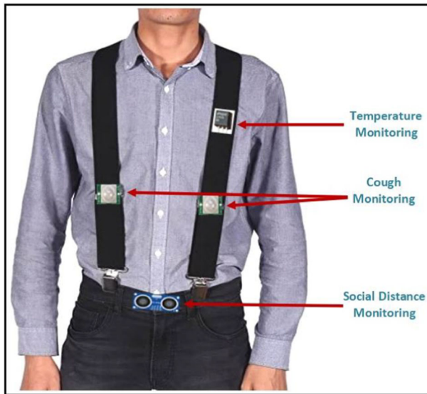
Fig. 6 Smart COVID-Shield embedded with suspender and belt
