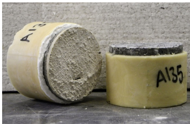
Fig. 28 Specimen of membrane M1 after shear testing exhibiting a debonding (adhesive) failure between membrane and the substrate concrete
