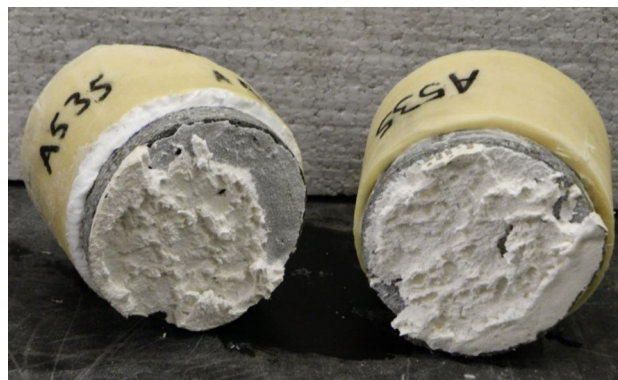
Fig. 30 Specimen of membrane M5 after shear testing exhibiting shear (cohesive) failure in the membrane material
