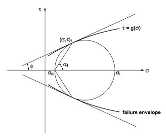
Fig. 1 Mohr diagram and failure envelopes
