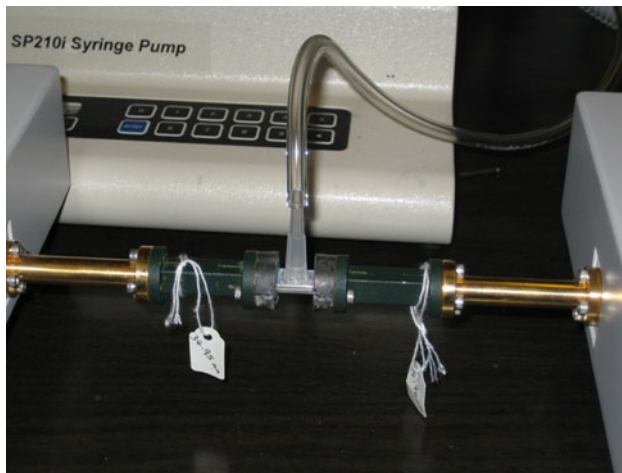
Fig. 6 Optical photo of the plastic tunable iris filter/phase shifter and experimental setup
