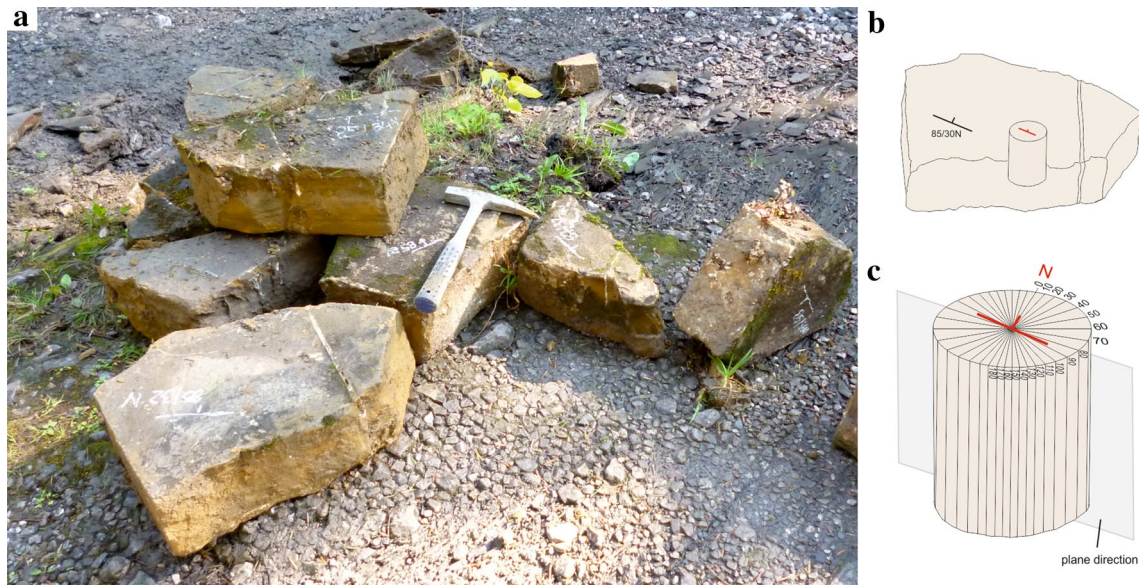
Fig. 4 Methodology of ultrasonic tests (Domonik 2007, modified): a rock monoliths from which the samples were cut to the laboratory tests; b orientation of cylindrical sample within rock monolith; c
