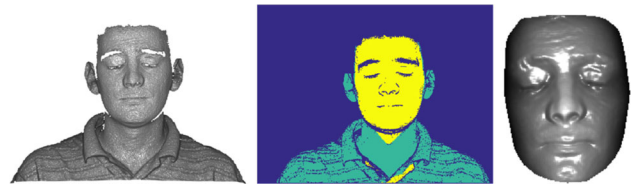
Fig. 7 Illustration of the face detection procedure used on the FRGCv2 and UND datasets. The procedure uses a simple k -means clustering approach (with k = 3 ) and selects the cluster with the lowest mean depth as the face region. The figure shows Input image (left), color coded clusters (middle), and cropped and smoothed face image (right)
