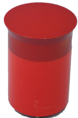
Fig. 3: Dummy for measuring the surface coverage of a single spread powder layer
