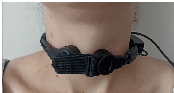
Fig. 1 Illustration of the skin-contact microphone
