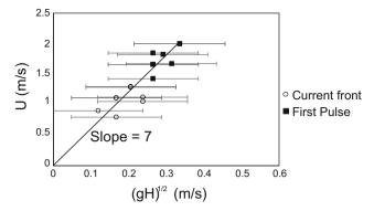
**Fig. 5** Froude number for the fronts and first pulses of selected experimental currents. Uncertainties in velocity are smaller than the size of the symbols. Uncertainties in current height are relatively large due to the thinness of the current fronts relative to video resolution
