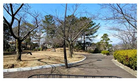
Fig. 4 Rolling shutter is a widely used shutter mechanism for mobile imaging. It induces artifacts, because the image is captured line by line. In this example, the pole appears unnaturally bent
