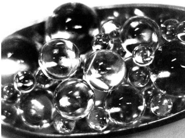
Fig. 3 Mixture of three different sizes of glass beads with diameters 2.5, 4.6 and 6.5 mm
