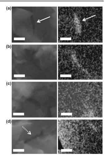
**Fig. 4** Comparison between small sections of SEM images (*left column*) and EUV images (*right column*) showing different areas of the sample. **a, b** Some cracks, as small as 100 nm, in the sample are deep all the way to the membrane and can be seen in both SEM and EUV images (marked with *white arrows* and **c, d** some of the features (marked with *dotted arrow*) are visible in the SEM images but are not present in the corresponding EUV image. *Scale bar* is 2 μm
