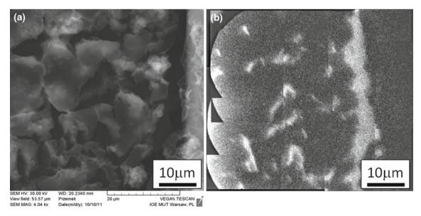
Fig. 3 SEM image of the sample,  $\sim 50 \times 50 \,\mu\text{m}^2$  with re-crystallized NaCl (a) and corresponding EUV image (b) showing the same region of the sample. EUV image was obtained by stitching and partially overlapping of  $4 \times 4$  smaller EUV sub-images
