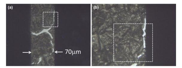
Fig. 2 Optical images of thin Si membrane with NaCl crystals deposited on top with a  $40 \times$  (NA = 0.65), b  $100 \times$  (NA ~ 1) objectives. Dashed boxes indicate the size of object region imaged with the EUV microscope
