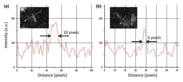
Fig. 5 Intensity profiles of smallest features in the EUV images (a) showing visible features as small as 4 pixel wide (b)
