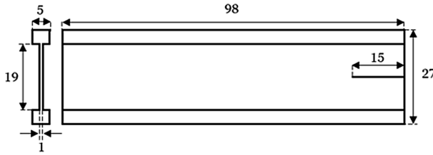
Fig. 2 Specimen used in pure shear fracture tests. Dimensions are expressed in mm
