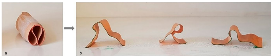
Fig. 1 Programming the initial state of beech veneer using its moisture content, a initial state of fully immersed wood, b time lapse showing its response through a duration of 3 min
