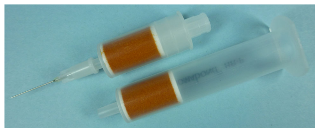
Fig. 1 Solid phase extraction (SPE) cartridges. Top : Solid phase extraction cartridge equipped for automated SPE. Bottom : Standard solid phase extraction cartridge
