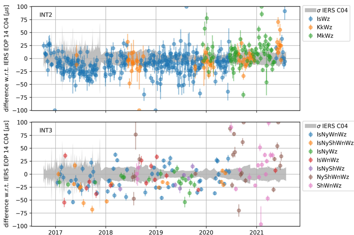
Fig. 6 Difference between estimated dUT1 values of GSF solution and IERS EOP 14 C04, color-coded by network. The IERS EOP 14 C04 dUT1 mean formal errors are depicted in gray. Top: INT2 baselines observed in at least 10 sessions. Bottom: INT3 networks observed in at least 5 sessions
