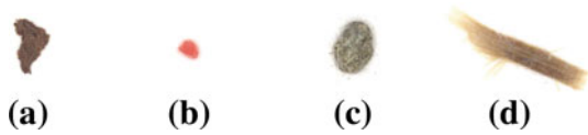
Fig. 2 Clearly different examples of the dirt particles: a bark, b plastic, c sand, d shive
