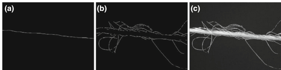
Fig. 14 Results of yarn components skeletonization: a skeleton of the yarn core, b skeletons of the protruding and looped fibres, c comparison of the skeletons and the original image
