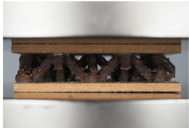
**Fig. 5** Sample of a sandwich panel during uniaxial compression
