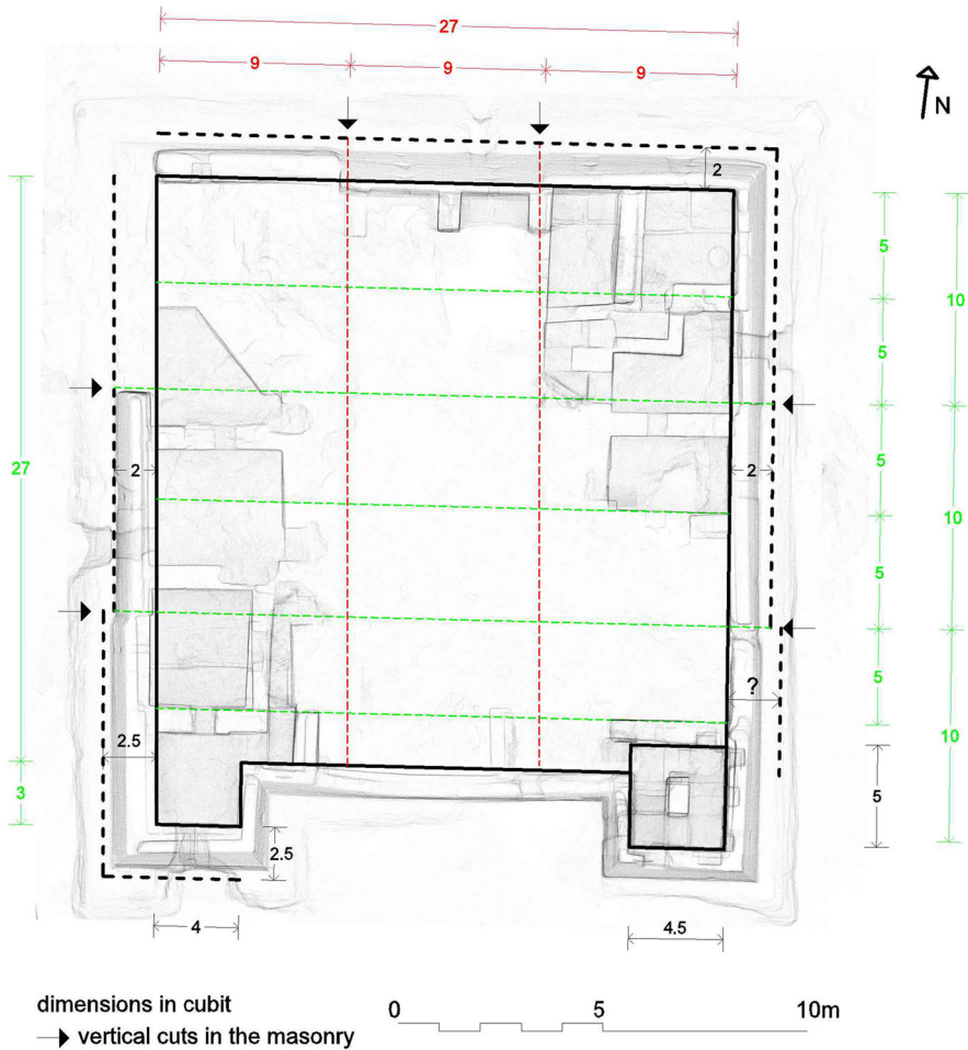
Fig. 10 Reconstruction of the geometrical scheme of the plan of the Fort, based on Egyptian cubits
