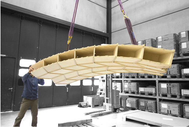
Fig. 2 Image from the paper “A Double-Layered Timber Plate Shell” presented at the AAG2016 conference. This 8 \times 7 segment prototype was fabricated from 15 mm birch veneer panels at a scale of 1:2.6. The completed prototype was exhibited during AAG2016. Photo: Laboratory for Timber Construction (IBOIS) and Computer Graphics and Geometry Laboratory (LGG), EPFL, 2016, reproduced by permission
