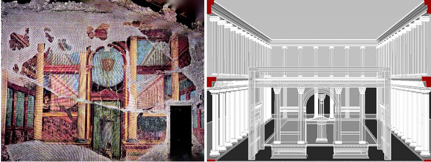
Fig. 4 Oplontis, villa of Poppaea: Salone , painted architecture ( left ) and perspective ( right ). Using the inverse perspective technique we can reach the geometric “reconstruction” of the drawn architectures. The virtual space that is rebuilt, is recomposed with the actual surveyed space, through plans, elevations and sections, adding more efficient representations such as perspectives and axonometric views that allow the experience of a brand new space to be captured. (Image processed by B. Messina)
