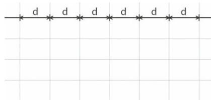
Fig. 1. The ideal length d defines equally spaced points along the horizontal direction
