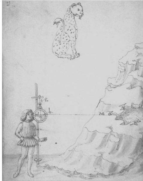
Fig. 5. Anonymous (da Taccola). Measurement of levels with an astrolabe. Ms. Palatino 767 (BNCF), p. 23
