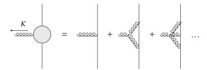
Figure 4. The matrix element of the stress-energy tensor  $\langle T_{\mu\nu}(K) \rangle$  corresponds to the 3 point function associated to a pair of massive particles and an external off-shell graviton. The coupling to internal gravitons emanating from the massive source yields, in the long-range behavior, higher corrections in G.
