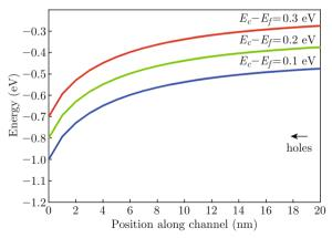
Fig. 4 Band diagrams of the CNTFETs with different Si doping level at the source side.
