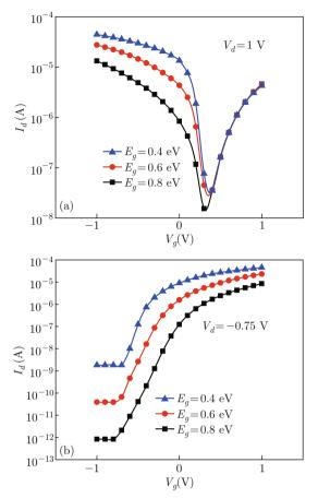
Fig. 5 Calculated transfer characteristics of the CNT-FETs with different SWNT band gaps for  $V_d = 1$  V (a) and  $V_d = -0.75$  V (b). The blue, red, and black curves are for  $E_g = 0.4$ , 0.6 and 0.8 eV, respectively.
