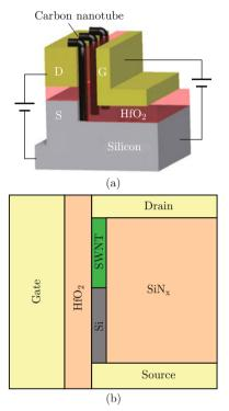
Fig. 1 a) 3D structure of the vertical CNTFET on silicon. b) Schematic configuration of the CNTFET for calculation. The vertical channel is composed of a SWNT and a Si nanowire.
