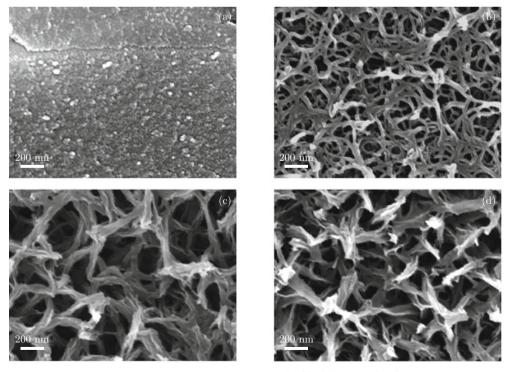
Fig. 3 SEM images of the films formed by treating Ti foils in  $H_2O_2(15\% v/v)$ -NaOH(2M) mixed solutions for 6 h at different temperatures: (a) 40°C, (b) 60°C, (c) 100°C, and (d) 120°C.
