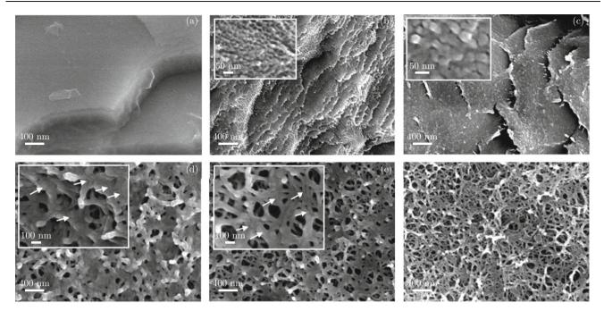
Fig. 5 SEM images of the films formed by treating Ti foils in  $H_2O_2(15\% v/v)$ -NaOH(2M) mixed solution at 80°C for different durations: (a) 0, (b) 0.5 h, (c) 1 h, (d) 1.5 h, (e) 2 h, and (f) 4 h. Insets of Fig. 5(b), 5(c), 5(d) and 5(e) are the high magnification images of corresponding materials.
