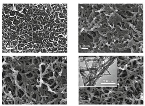
Fig. 1 SEM images of the films formed by treating Ti foils at 80°C for 6 h in H<sub>2</sub>O<sub>2</sub>-NaOH(2M) mixed solutions with different H<sub>2</sub>O<sub>2</sub> concentrations. (a) 0, (b) 7.5% v/v, (c) 11.25% v/v, and (d) 15% v/v. Inset of Fig. 2(d) is the corresponding TEM image of the nanowires.
