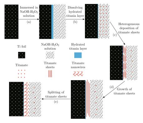
Fig. 6 A scheme for the formation of titanate nanowires films in NaOH-H<sub>2</sub>O<sub>2</sub> aqueous solutions.
