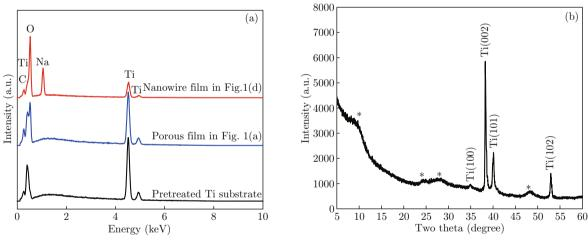
Fig. 2 (a) EDS spectra of pretreated Ti substrate, porous film formed in NaOH solution, and nanowire film formed in H<sub>2</sub>O<sub>2</sub>-NaOH mixed solution, and (b) XRD pattern of the nanowire film formed by treating Ti foils in H<sub>2</sub>O<sub>2</sub>(15%v/v)-NaOH(2M) mixed solutions for 6 h at 80°C.
