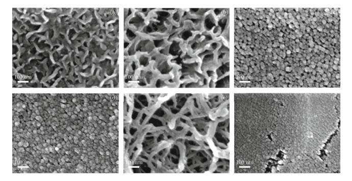
Fig. 4 SEM images of the films formed by treating Ti foils at 80°C for 6 h in different solutions with the concentration of  $H_2O_2$  being fixed at 15% v/v: (a)  $NaCl(2M)-H_2O_2$ , (b)  $H_2O_2$ , (c)  $NH_3 \cdot H_2O(18.5\% v/v)-H_2O_2$ , (d)  $NaCl(2M)-NH_3 \cdot H_2O(18.5\% v/v)-H_2O_2$ , (e)  $KOH(2M)-H_2O_2$ , and (f)  $Ba(OH)_2(1.5M)-H_2O_2$ .
