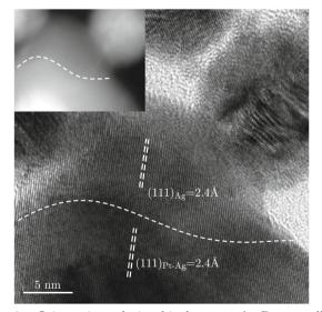
Fig. 3 Orientation relationship between Ag-Pt nanoalloy and Ag nano-brazing filler metal, showing the minimum interfacial mismatch.
