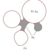
Fig. 2 STEM image of nano brazed joint by femtosecond laser irradiation. The nano Ag cluster was the filler metal and Pt-Ag nanoalloy was the base metal.
