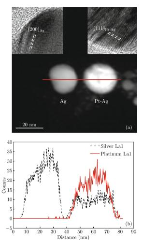
Fig. 1 Typical Ag and Pt-Ag nanoparticles: (a) STEM of isolated Ag and Pt-Ag nanoparticles, the lattice spacing of  $(200)_{Ag}$  was 2.09 Å and  $(111)_{Pt-Ag}$  was 2.33 Å; (b) EDS line scan in (a).
