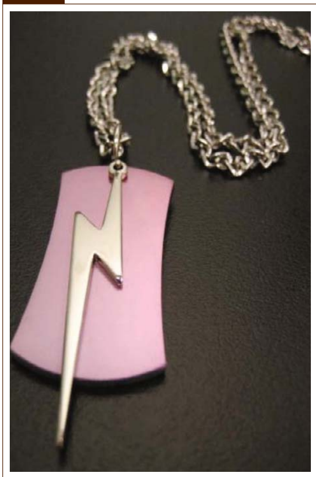
Prototype item of stainless steel costume jewellery onto which a film of \text{AuAl}_2 of about 200 nm thickness has been applied for decorative effect
