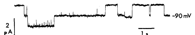
Fig. 1. Channel activity observed in an inside-out patch with 140 mM NaCl, 1 mM \text{CaCl}_2 , 1 mM \text{MgCl}_2 in the pipette and 140 mM KCl, 1 mM EGTA, 1 mM \text{MgCl}_2 in the bath. Both solutions were buffered with 1 mM Tris-Cl to pH 7.4.
